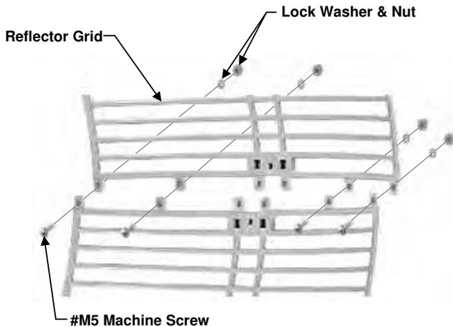
Assemble the halves of the Reflector Grid using (4) #M5 machine screws with lock washers, flat washers and nuts as shown.
