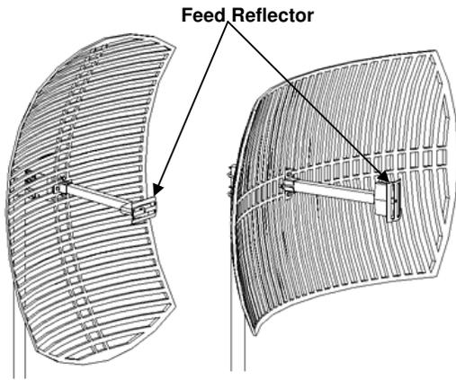
**Important Note:** Feed Reflector must be orientated to grid as shown for optimal antenna performance.
