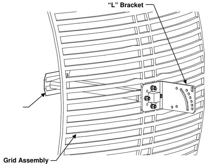
Install the (2) Mast Clamps on the U-Bolts as shown and fasten to the "L" Bracket using (4) lock washers and (4) Nuts.
