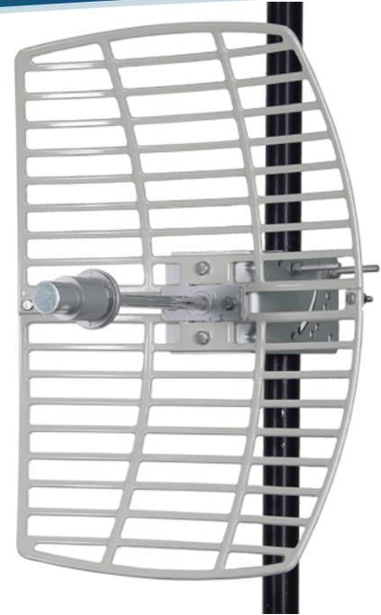
Assemble the halves of the Reflector Grid using (2) #M5 machine screws with lock washers, flat washers and nuts as shown.
